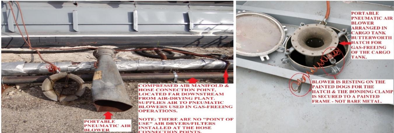
**Not installing "point of use" air dryers/filters at hose connection points for pneumatic air blowers (left photo) & attaching air blower bonding clamps to painted surfaces instead of bare metal (right photo) can lead to dangerous static build up.**
