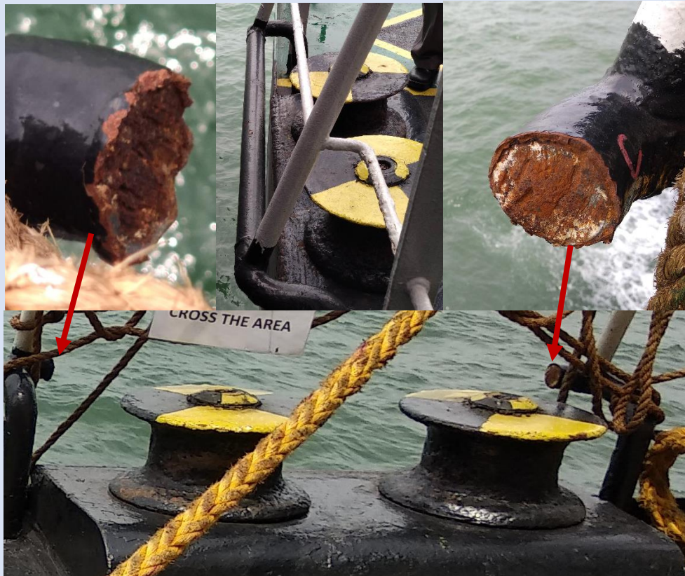
Figure 1: The sheared off “stopper bar” above the roller fairleads
