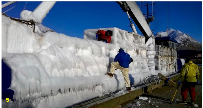
Ice accumulation on vessels operating near the capsized vessel Destination that was lost in the Bering Sea. (4) Bering Rose : accumulation of ice on deck aft of the wheelhouse on February 11. (5) Sandra Five : crewmembers examine ice while in King Cove, Alaska, on February 12.
