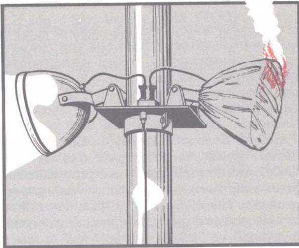
The heat of the lamp can ignite covers left in place over floodlights.
