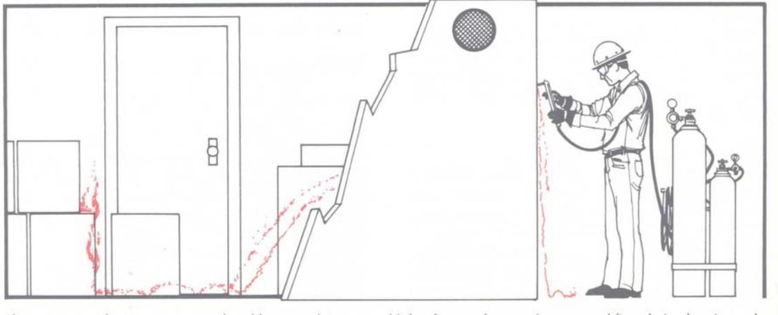
Failure to remove combustible materials or to establish a fire watch may be factors in fires ignited during burning and welding operations.
