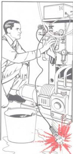
An unprotected droplight bulb can easily break, allowing the live electric circuit to ignite nearby flammable material.
