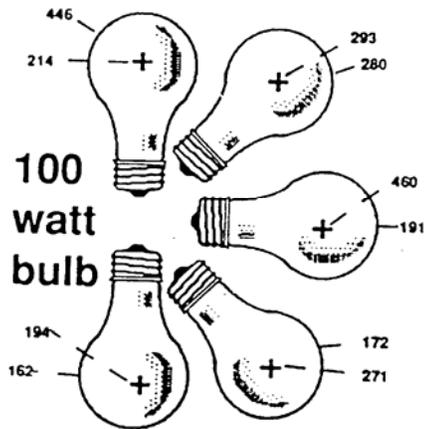
This diagram shows the various hotspots of a light bulb mounted in various positions. Note that when a light bulb is mounted in the upright position, the tip of the light bulb
