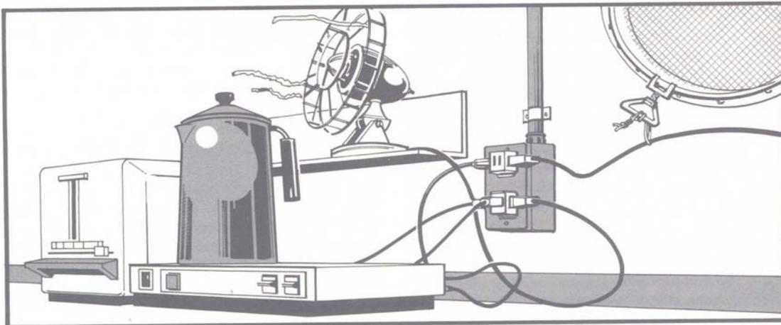
Overloading is dangerous. Only one appliance should be connected to each outlet in an electric circuit.
