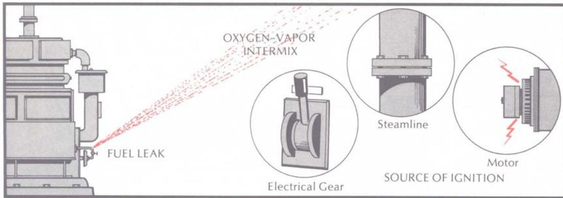
Fuel line leaks can spray vaporized fuel far enough to be ignited by steam lines or electrical equipment located nearby.
