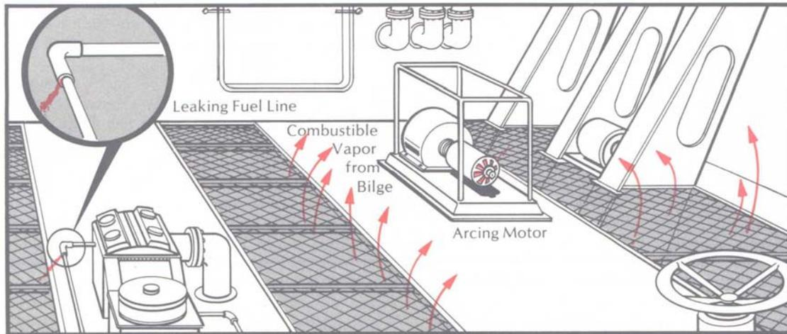
Fuel from leaking oil line collects in the bilge. Combustible fuel vapors from the bilge mix with air as they move toward the arcing motor. Ignition of the fumes by the motor can cause an explosion followed by fire.
